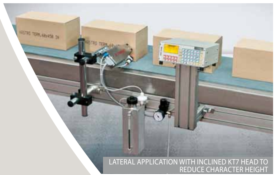
LATERAL AND VERTICAL APPLICATION WITH TWO KT7 HEADS
